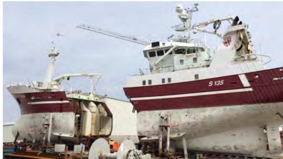
Split ready for lengthening at Karstensens Shipyard.
