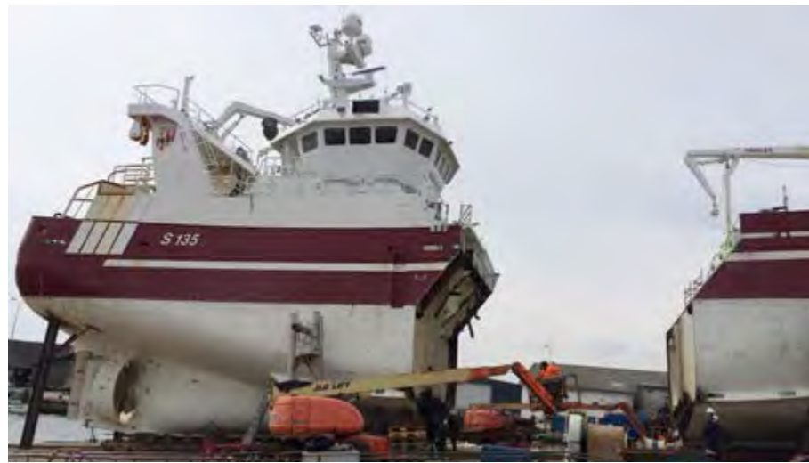
Split ready for lengthening at Karstensens Shipyard.
