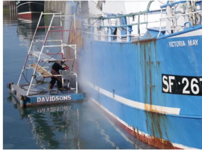
Pressure washing before lifting out.
